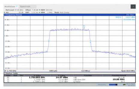
LTE band 66, 20MHz Bandwidth, MID, 16QAM (-26dBc BW)
