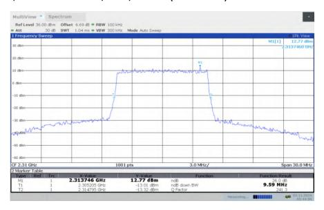
LTE band 30, 10MHz Bandwidth, LOW, 64QAM (-26dBc BW)
