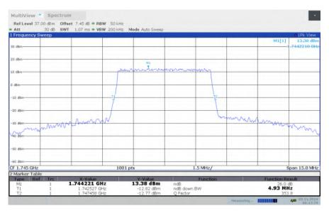
LTE band 66, 5MHz Bandwidth, MID, 16QAM (-26dBc BW)
