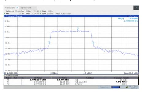
LTE band 41, 5MHz Bandwidth, LOW, 16QAM (-26dBc BW)
