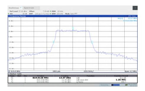
LTE band 26, 1.4MHz Bandwidth, MID, 64QAM (-26dBc BW)
