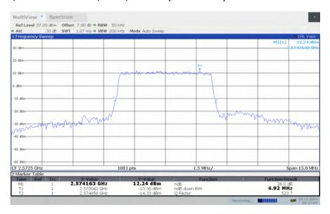
LTE band 38, 5MHz Bandwidth, LOW, 64QAM (-26dBc BW)
