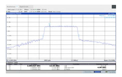
LTE band 41, 5MHz Bandwidth, MID, 64QAM (-26dBc BW)
