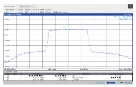
LTE band 26, 10MHz Bandwidth, HIGH, 64QAM (-26dBc BW)
