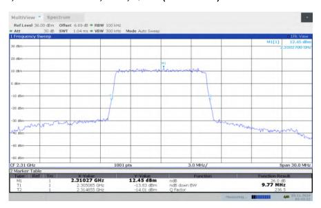
LTE band 30, 10MHz Bandwidth, LOW, 16QAM (-26dBc BW)
