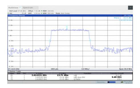
LTE band 38, 10MHz Bandwidth, HIGH, 16QAM (-26dBc BW)
