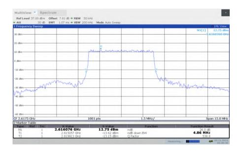
LTE band 38, 5MHz Bandwidth, HIGH, 16QAM (-26dBc BW)
