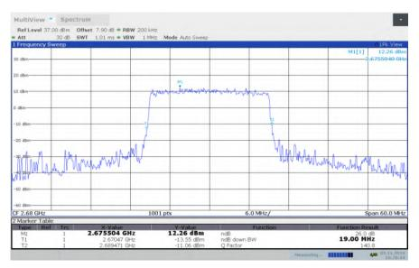
LTE band 41, 20MHz Bandwidth, HIGH, 64QAM (-26dBc BW)
