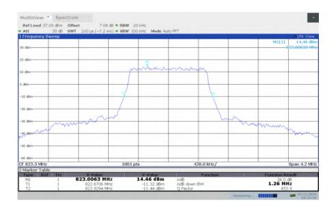
LTE band 26, 1.4MHz Bandwidth, HIGH, 16QAM (-26dBc BW)
