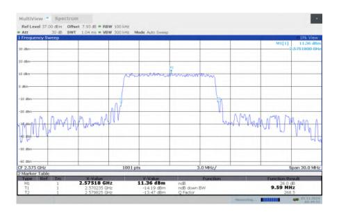
LTE band 38, 10MHz Bandwidth, MID, QPSK (-26dBc BW)
