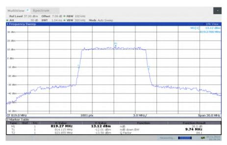
LTE band 26, 10MHz Bandwidth, MID, 16QAM (-26dBc BW)
