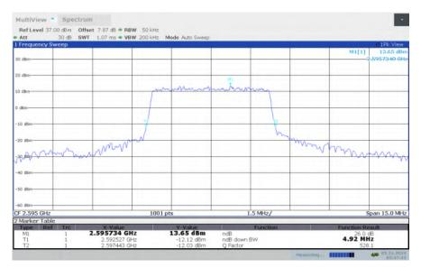
LTE band 38, 5MHz Bandwidth, MID, 16QAM (-26dBc BW)
