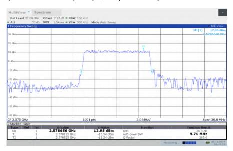
LTE band 38, 10MHz Bandwidth, LOW, 16QAM (-26dBc BW)
