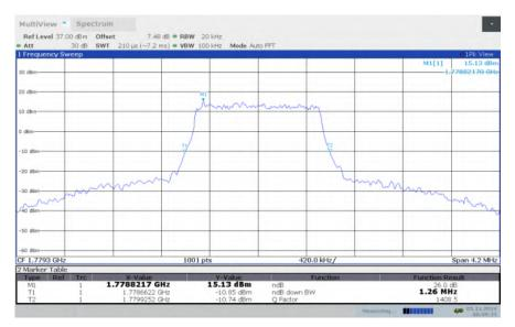
LTE band 66, 1.4MHz Bandwidth, HIGH, 64QAM (-26dBc BW)
