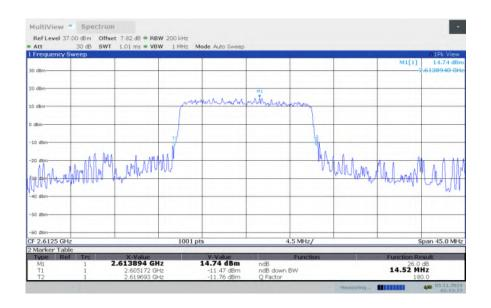
LTE band 38, 15MHz Bandwidth, HIGH, 16QAM (-26dBc BW)
