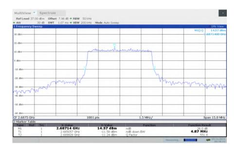
LTE band 41, 5MHz Bandwidth, HIGH, 16QAM (-26dBc BW)
