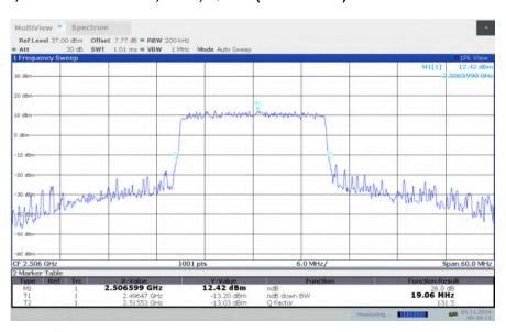
LTE band 41, 20MHz Bandwidth, LOW, 16QAM (-26dBc BW)
