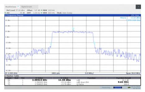
LTE band 38, 10MHz Bandwidth, HIGH, QPSK (-26dBc BW)
