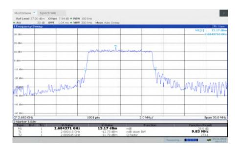
LTE band 41, 10MHz Bandwidth, HIGH, 16QAM (-26dBc BW)
