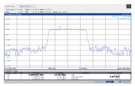
LTE band 41, 10MHz Bandwidth, HIGH, 64QAM (-26dBc BW)
