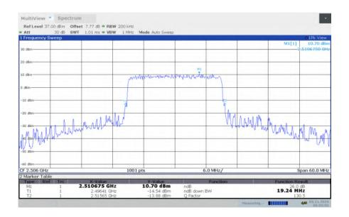
LTE band 41, 20MHz Bandwidth, MID, QPSK (-26dBc BW)
