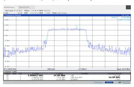
LTE band 41, 15MHz Bandwidth, LOW, 16QAM (-26dBc BW)
