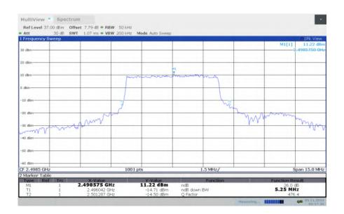
LTE band 41, 5MHz Bandwidth, MID, QPSK (-26dBc BW)
