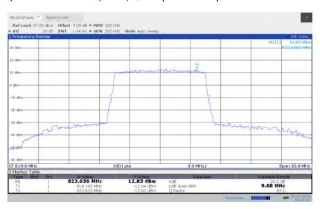
LTE band 26, 10MHz Bandwidth, LOW, 16QAM (-26dBc BW)
