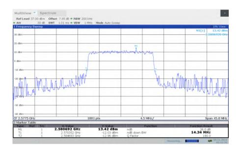
LTE band 38, 15MHz Bandwidth, MID, QPSK (-26dBc BW)
