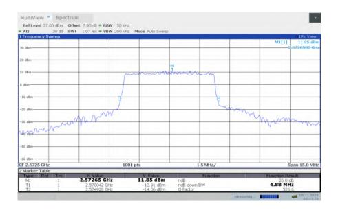
LTE band 38, 5MHz Bandwidth, MID, QPSK (-26dBc BW)
