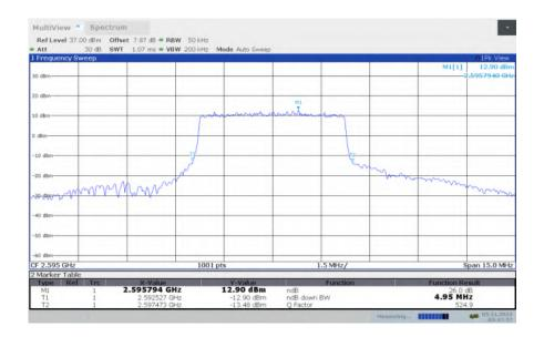
LTE band 38, 5MHz Bandwidth, MID, 64QAM (-26dBc BW)
