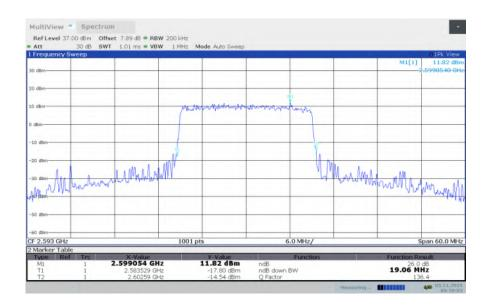
LTE band 41, 20MHz Bandwidth, MID, 64QAM (-26dBc BW)
