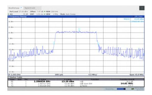
LTE band 38, 15MHz Bandwidth, MID, 64QAM (-26dBc BW)
