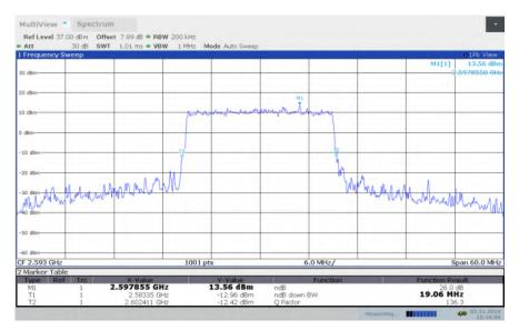
LTE band 41, 20MHz Bandwidth, MID, 16QAM (-26dBc BW)
