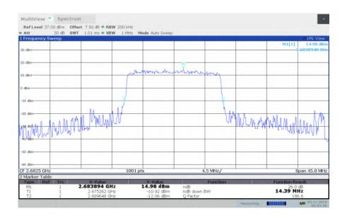
LTE band 41, 15MHz Bandwidth, HIGH, 16QAM (-26dBc BW)
