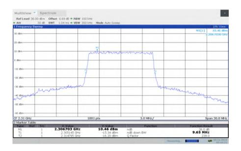
LTE band 30, 10MHz Bandwidth, MID, QPSK (-26dBc BW)
