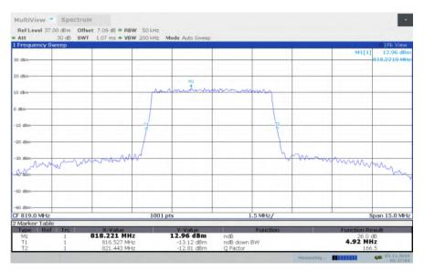
LTE band 26, 5MHz Bandwidth, MID, 16QAM (-26dBc BW)
