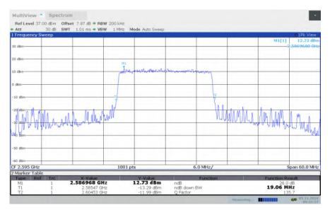
LTE band 38, 20MHz Bandwidth, MID, 16QAM (-26dBc BW)
