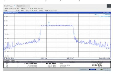
LTE band 41, 20MHz Bandwidth, LOW, 64QAM (-26dBc BW)
