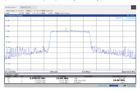
LTE band 38, 20MHz Bandwidth, LOW, 64QAM (-26dBc BW)
