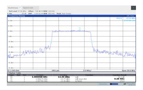
LTE band 41, 10MHz Bandwidth, MID, 64QAM (-26dBc BW)
