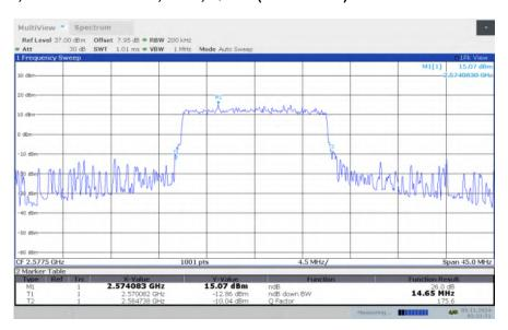
LTE band 38, 15MHz Bandwidth, LOW, 16QAM (-26dBc BW)
