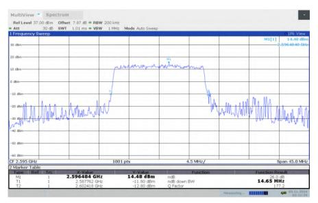
LTE band 38, 15MHz Bandwidth, MID, 16QAM (-26dBc BW)
