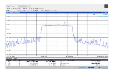
LTE band 38, 20MHz Bandwidth, MID, QPSK (-26dBc BW)
