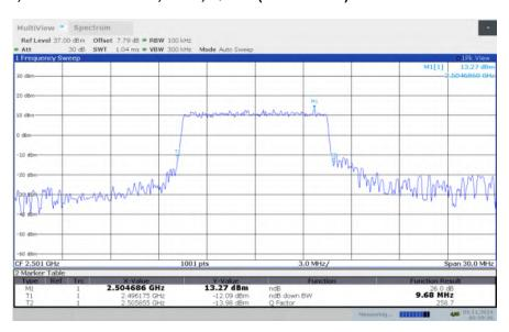
LTE band 41, 10MHz Bandwidth, LOW, 16QAM (-26dBc BW)
