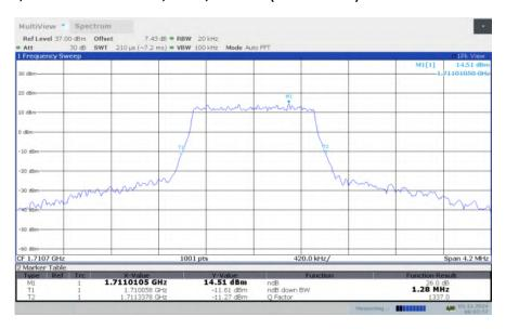
LTE band 66, 1.4MHz Bandwidth, LOW, 64QAM (-26dBc BW)
