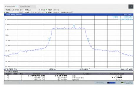
LTE band 66, 1.4MHz Bandwidth, LOW, 16QAM (-26dBc BW)
