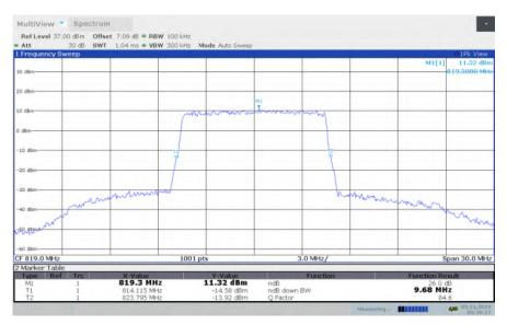
LTE band 26, 10MHz Bandwidth, HIGH, QPSK (-26dBc BW)
