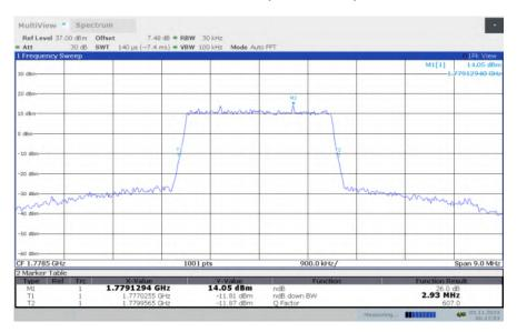
LTE band 66, 3MHz Bandwidth, HIGH, 64QAM (-26dBc BW)
