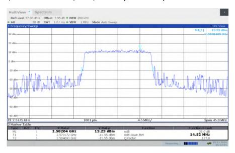
LTE band 38, 15MHz Bandwidth, LOW, 64QAM (-26dBc BW)
