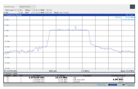
LTE band 38, 5MHz Bandwidth, LOW, 16QAM (-26dBc BW)
