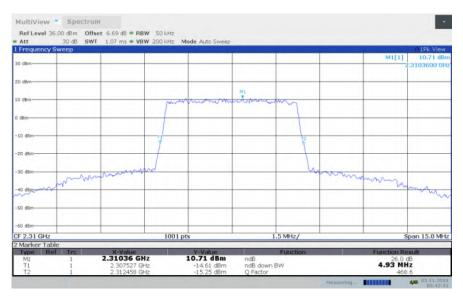
LTE band 30, 5MHz Bandwidth, HIGH, QPSK (-26dBc BW)
