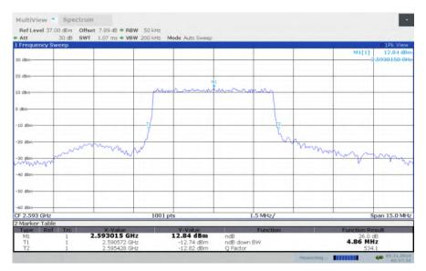
LTE band 41, 5MHz Bandwidth, MID, 16QAM (-26dBc BW)
