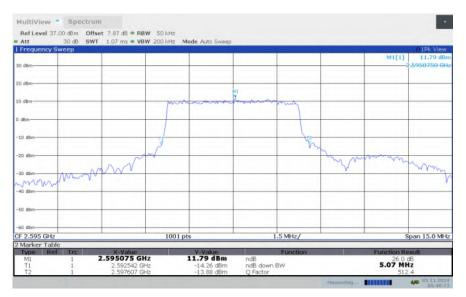
LTE band 38, 5MHz Bandwidth, HIGH, QPSK (-26dBc BW)
