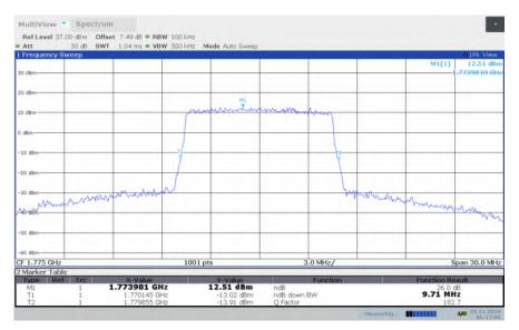
LTE band 66, 10MHz Bandwidth, HIGH, 64QAM (-26dBc BW)
