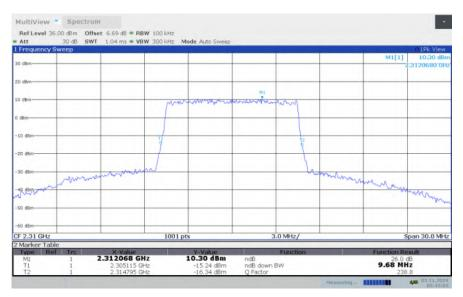
LTE band 30, 10MHz Bandwidth, HIGH, QPSK (-26dBc BW)
