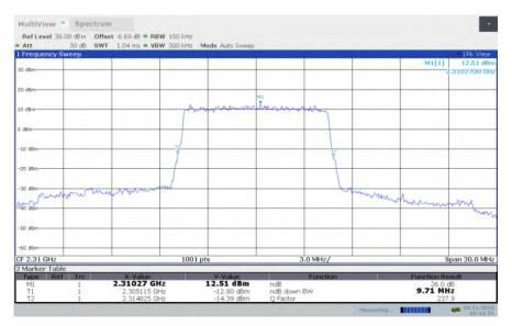
LTE band 30, 10MHz Bandwidth, MID, 16QAM (-26dBc BW)
