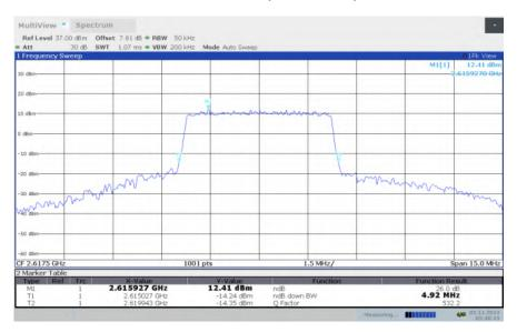
LTE band 38, 5MHz Bandwidth, HIGH, 64QAM (-26dBc BW)
