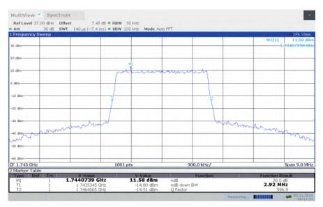
LTE band 66, 3MHz Bandwidth, HIGH, QPSK (-26dBc BW)
