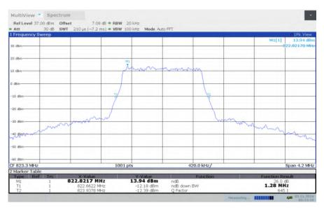
LTE band 26, 1.4MHz Bandwidth, HIGH, 64QAM (-26dBc BW)
