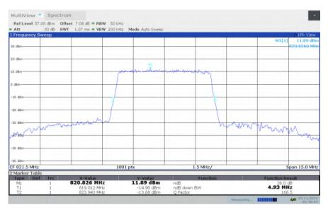
LTE band 26, 5MHz Bandwidth, HIGH, 64QAM (-26dBc BW)
