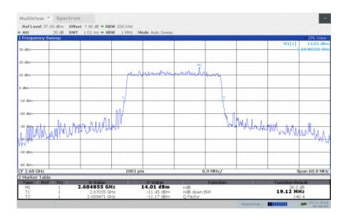
LTE band 41, 20MHz Bandwidth, HIGH, 16QAM (-26dBc BW)
