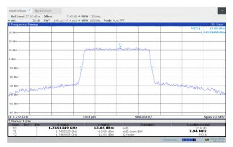
LTE band 66, 3MHz Bandwidth, MID, 16QAM (-26dBc BW)
