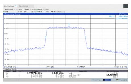
LTE band 66, 15MHz Bandwidth, HIGH, 64QAM (-26dBc BW)
