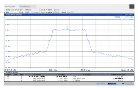
LTE band 26, 1.4MHz Bandwidth, HIGH, QPSK (-26dBc BW)
