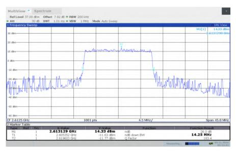
LTE band 38, 15MHz Bandwidth, HIGH, 64QAM (-26dBc BW)
