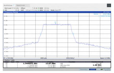
LTE band 66, 1.4MHz Bandwidth, HIGH, QPSK (-26dBc BW)
