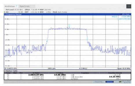
LTE band 41, 15MHz Bandwidth, HIGH, 64QAM (-26dBc BW)
