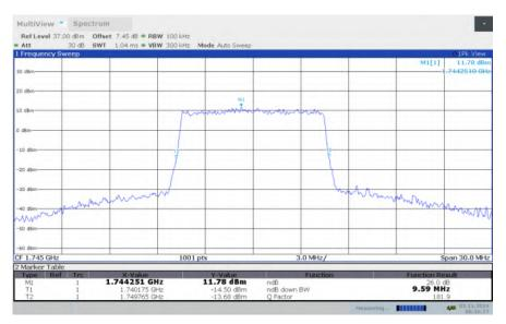
LTE band 66, 10MHz Bandwidth, HIGH, QPSK (-26dBc BW)
