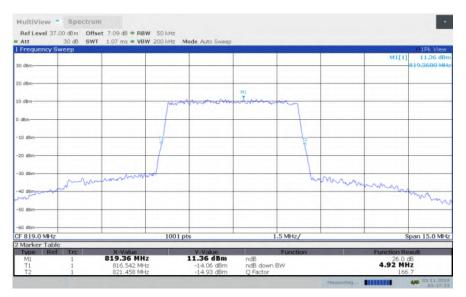
LTE band 26, 5MHz Bandwidth, HIGH, QPSK (-26dBc BW)
