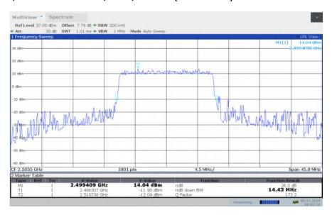
LTE band 41, 15MHz Bandwidth, LOW, 64QAM (-26dBc BW)
