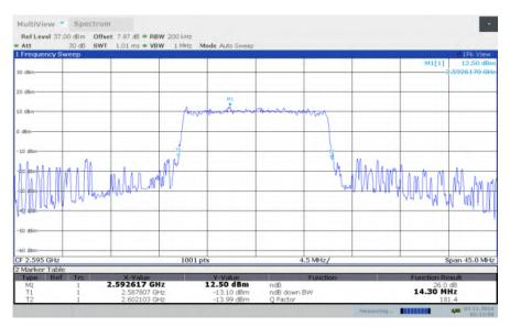
LTE band 38, 15MHz Bandwidth, HIGH, QPSK (-26dBc BW)
