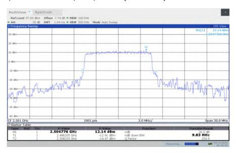
LTE band 41, 10MHz Bandwidth, LOW, 64QAM (-26dBc BW)
