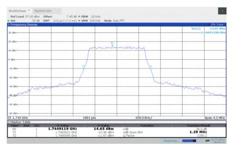
LTE band 66, 1.4MHz Bandwidth, MID, 16QAM (-26dBc BW)
