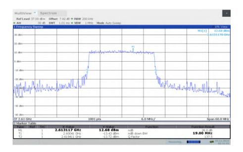
LTE band 38, 20MHz Bandwidth, HIGH, 16QAM (-26dBc BW)
