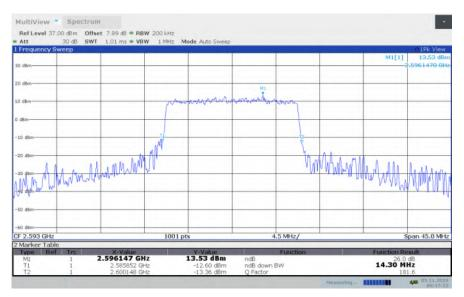
LTE band 41, 15MHz Bandwidth, HIGH, QPSK (-26dBc BW)
