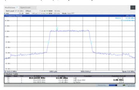
LTE band 26, 3MHz Bandwidth, LOW, 16QAM (-26dBc BW)
