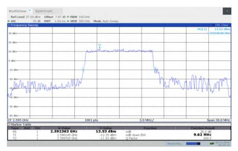
LTE band 38, 10MHz Bandwidth, MID, 16QAM (-26dBc BW)
