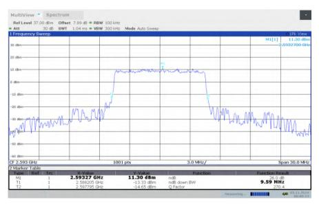
LTE band 41, 10MHz Bandwidth, HIGH, QPSK (-26dBc BW)
