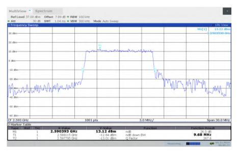
LTE band 41, 10MHz Bandwidth, MID, 16QAM (-26dBc BW)
