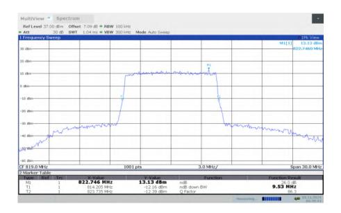
LTE band 26, 10MHz Bandwidth, MID, 64QAM (-26dBc BW)
