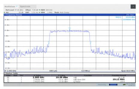
LTE band 41, 20MHz Bandwidth, HIGH, QPSK (-26dBc BW)
