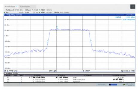
LTE band 66, 5MHz Bandwidth, HIGH, 64QAM (-26dBc BW)
