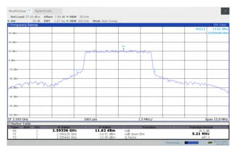
LTE band 41, 5MHz Bandwidth, HIGH, QPSK (-26dBc BW)
