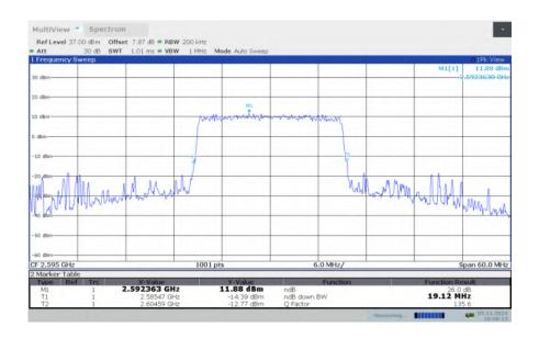
LTE band 38, 20MHz Bandwidth, MID, 64QAM (-26dBc BW)
