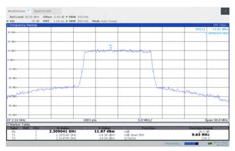
LTE band 30 , 10MHz Bandwidth, HIGH, 64QAM (-26dBc BW)
