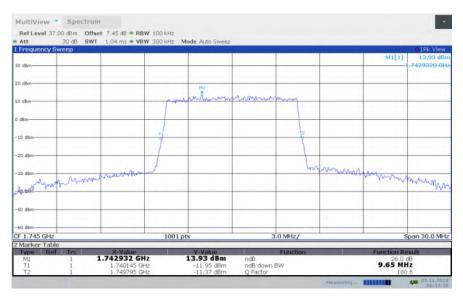
LTE band 66, 10MHz Bandwidth, MID, 16QAM (-26dBc BW)
