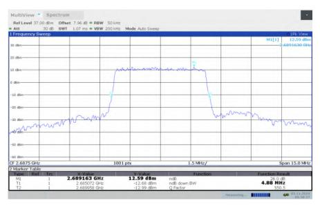
LTE band 41, 5MHz Bandwidth, HIGH, 64QAM (-26dBc BW)
