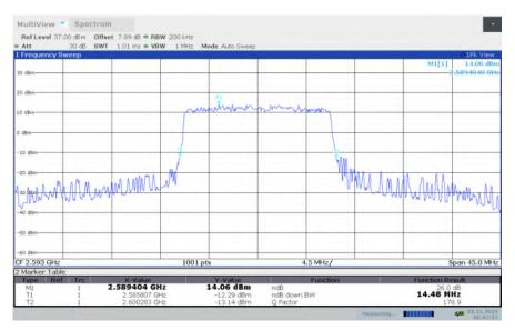
LTE band 41, 15MHz Bandwidth, MID, 16QAM (-26dBc BW)
