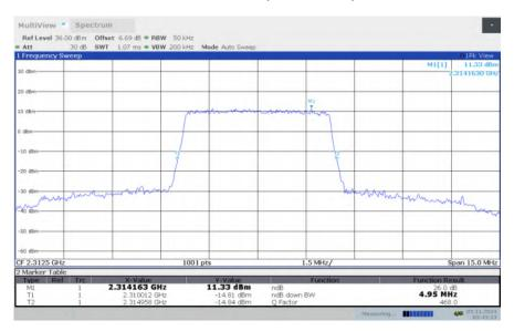
LTE band 30, 5MHz Bandwidth, HIGH, 64QAM (-26dBc BW)
