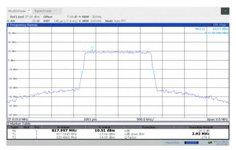
LTE band 26, 3MHz Bandwidth, HIGH, QPSK (-26dBc BW)
