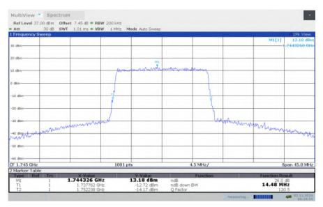
LTE band 66, 15MHz Bandwidth, HIGH, QPSK (-26dBc BW)
