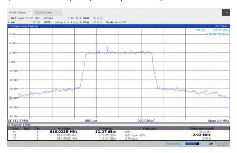
LTE band 26, 3MHz Bandwidth, LOW, 64QAM (-26dBc BW)
