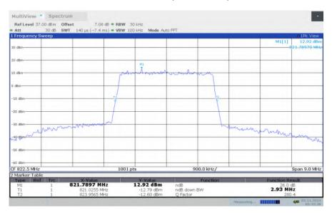
LTE band 26, 3MHz Bandwidth, HIGH, 64QAM (-26dBc BW)
