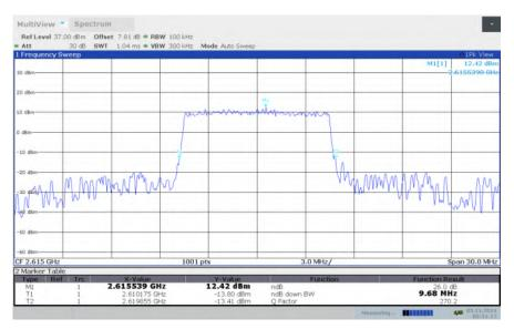
LTE band 38, 10MHz Bandwidth, HIGH, 64QAM (-26dBc BW)
