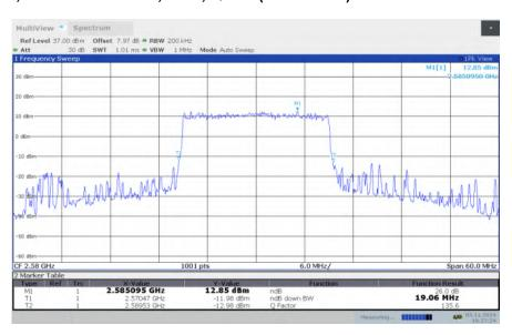
LTE band 38, 20MHz Bandwidth, LOW, 16QAM (-26dBc BW)
