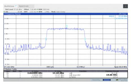
LTE band 38, 20MHz Bandwidth, HIGH, 64QAM (-26dBc BW)
