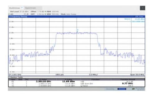
LTE band 41, 10MHz Bandwidth, MID, QPSK (-26dBc BW)
