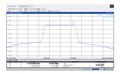
LTE band 30, 10MHz Bandwidth, MID, 64QAM (-26dBc BW)
