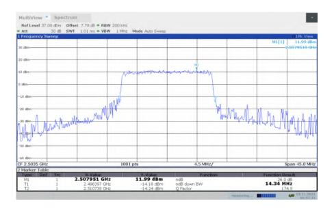
LTE band 41, 15MHz Bandwidth, MID, QPSK (-26dBc BW)
