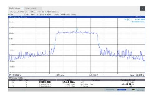
LTE band 41, 15MHz Bandwidth, MID, 64QAM (-26dBc BW)
