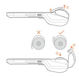
This device can load a 58mm thermal receipt or label paper roll.
