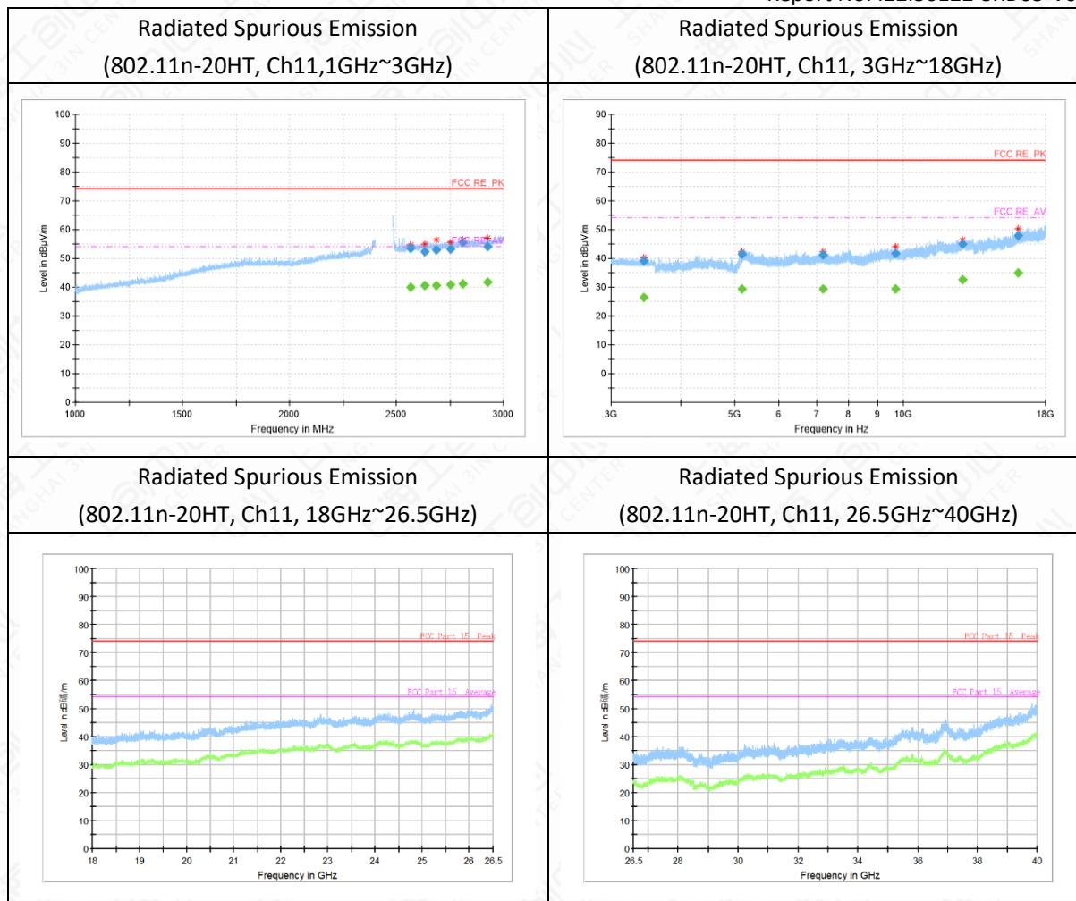
Note: The out-of-limit signal in the picture is the main frequency signal.
