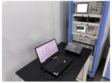
Radiated Spurious Emissions 9kHz-30MHz
