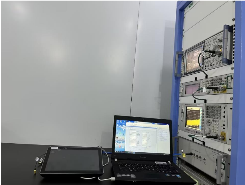
RF Conducted Test Setup
