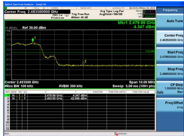
BT 3DH5 CH78, Carrier frequency (MHz): 2480
