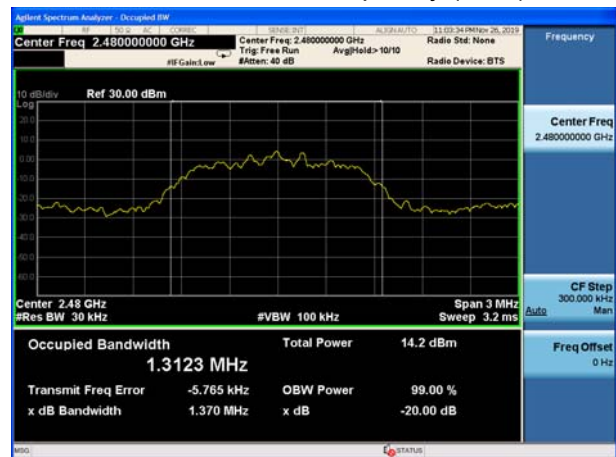
BT 2DH5 CH78, Carrier frequency (MHz): 2480
