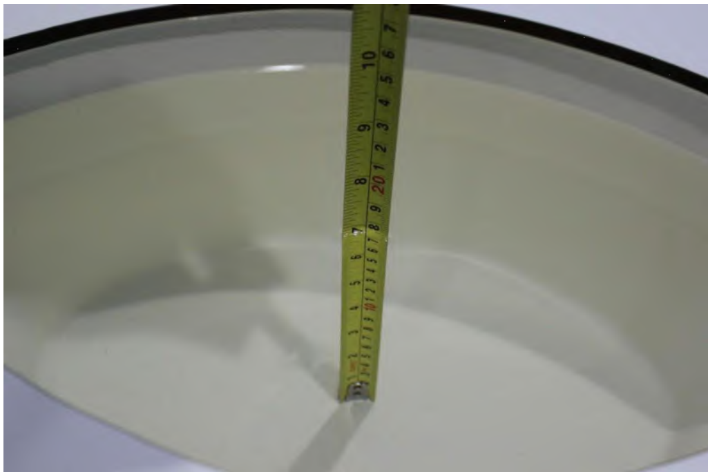
Picture 7-8: Liquid depth in the Flat Phantom (5GHz)
