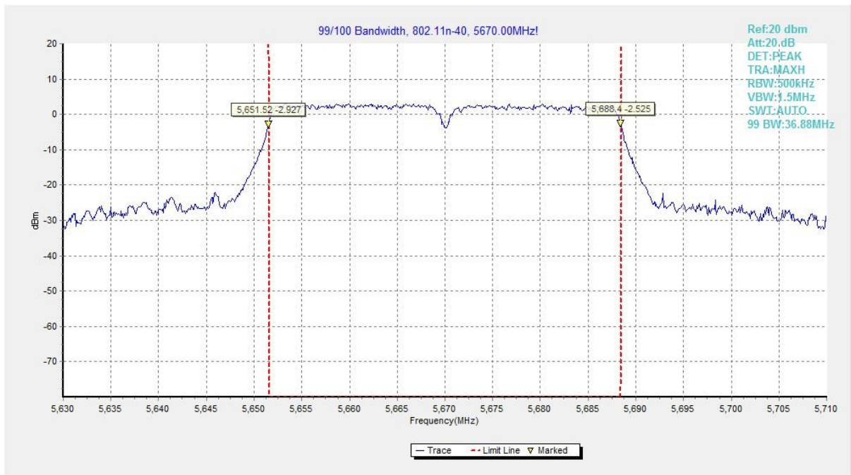
Fig. 42 99% Occupied Bandwidth (802.11n-HT40, 5670MHz)
