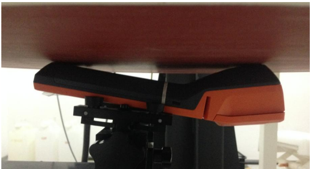
POSITION OF BODY BACK WITH 0mm DISTANCE
