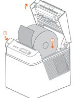
1) Press the door cover button to open the printer flip cover.
