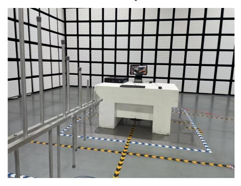
Front view of Radiated Emission Test Setup (Below 1GHz)
