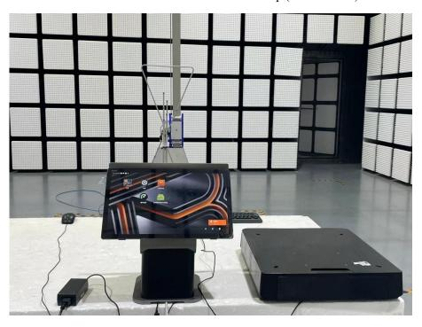
Back view of Radiated Emission Test Setup (Below 1GHz)
