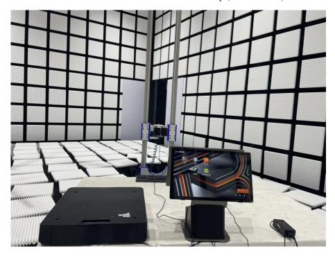
Back view of Radiated Emission Test Setup (Above 1GHz)
