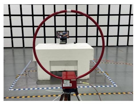
Front view of Field Radiated Emissions (Below 30MHz)
