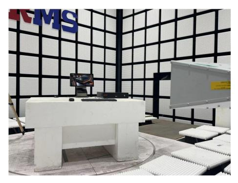
Front view of Radiated Emission Test Setup (Above 1GHz)
