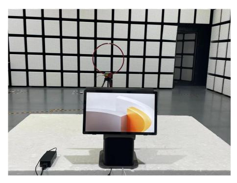
Back view of Field Radiated Emissions (Below 30MHz)
