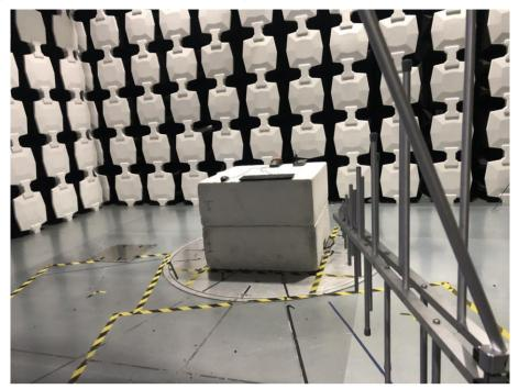
Description: Radiated Emission Test Setup
