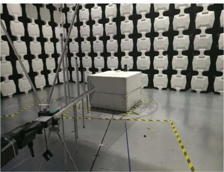
Description: Radiated Emission Test Setup
