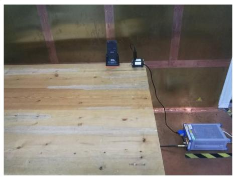
Test Mode: Mode 1 Description: Conducted Emission Test Setup
