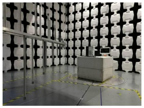
Description: Radiated Emission Test Setup
