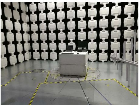
Description: Radiated Emission Test Setup
