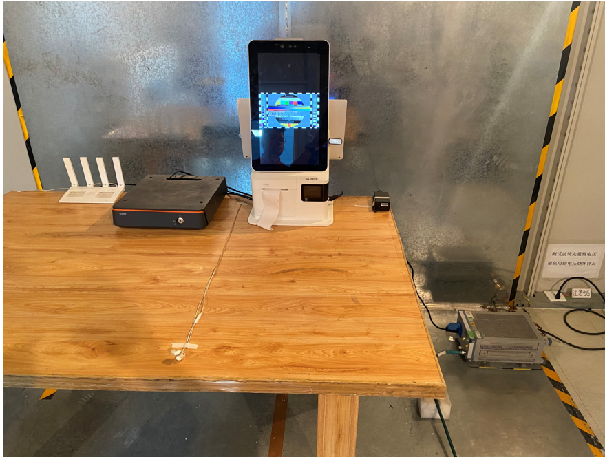
Conducted Emissions - Rear Side
