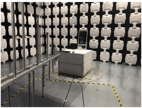
Description: Radiated Emission Test Setup
