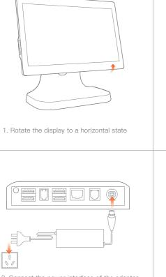
3. Connect the power interface of the adapter to the power port at the bottom of the mainframe. And insert the other side of the adapter to electric supply sockets
