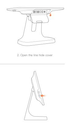
4. Press the power button for two seconds to turn on.
