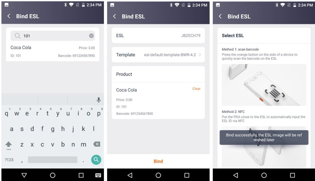
After completing the binding of all products and ESL, return to the home page of the SUNMI ESL APP. When the number of ESLs to be pushed becomes 0, that means all the ESLs are completed and the ESL system is deployed for the first time.
