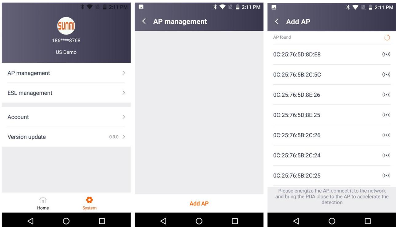
3. Select the access point that needs to be added (according to the signal strength or MAC address, the scanned MAC address is the same as the MAC address on the bottom nameplate of the access point) to enter the process of the access point adding and configuring.
