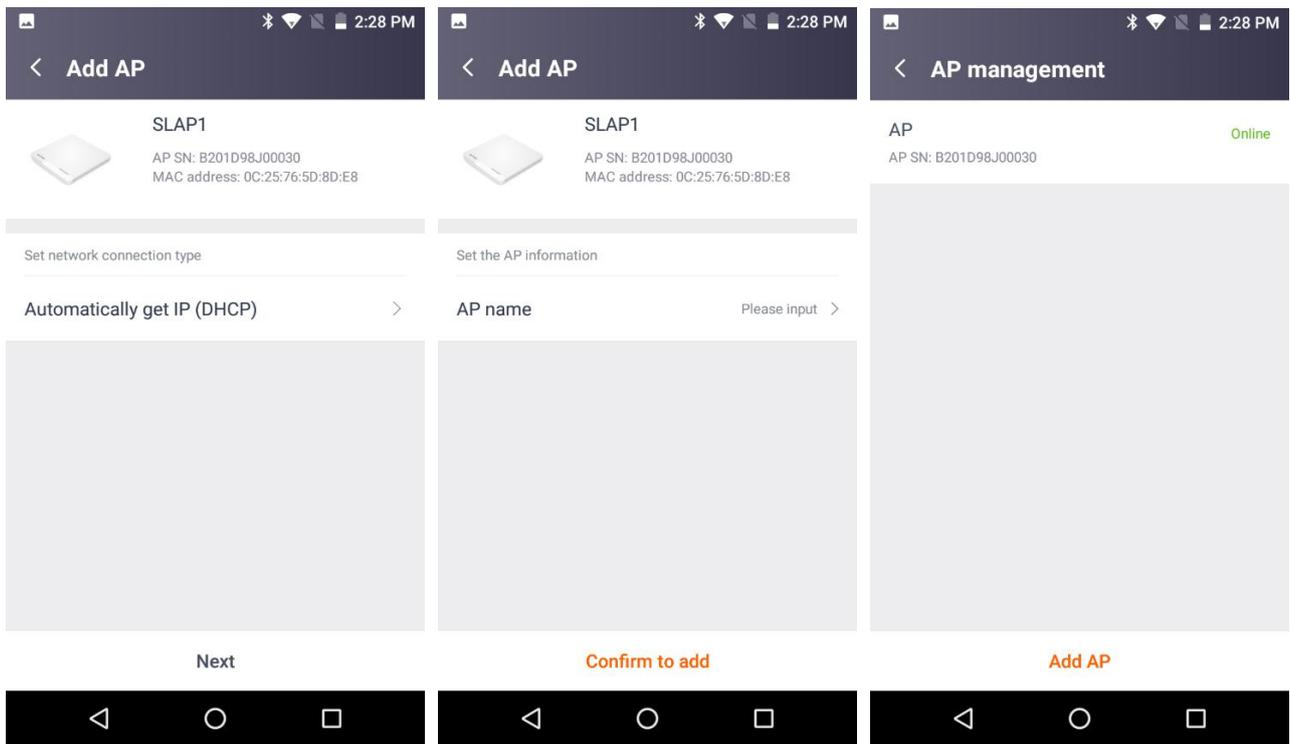
When the access point configuration is completed, the added access point will be seen in the access point list, and if the access point status is online, it is in normal operate. If the access point is offline, please check the connection status of power supply and the network, and try to reconfigure the access point access mode.
