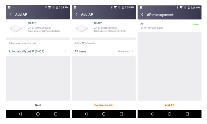
When the access point configuration is completed, the added access point will be seen in the access point list, and if the access point status is online, it is in normal operate. If the access point is offline, please check the connection status of power supply and the network, and try to reconfigure the access point access mode.
