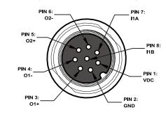
This connector is available on models BIS U-620-068-1x1-00-S29. See the BIS U-62 Processor Manual for details
