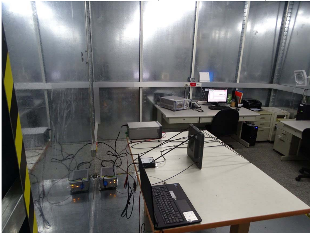
Back View of Conducted Test (BIS U-620-068-111-00-S115)
