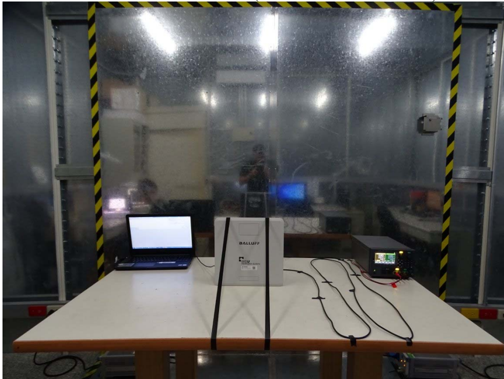
Front View of Conducted Test (BIS U-626-069-111-06-ST32)
