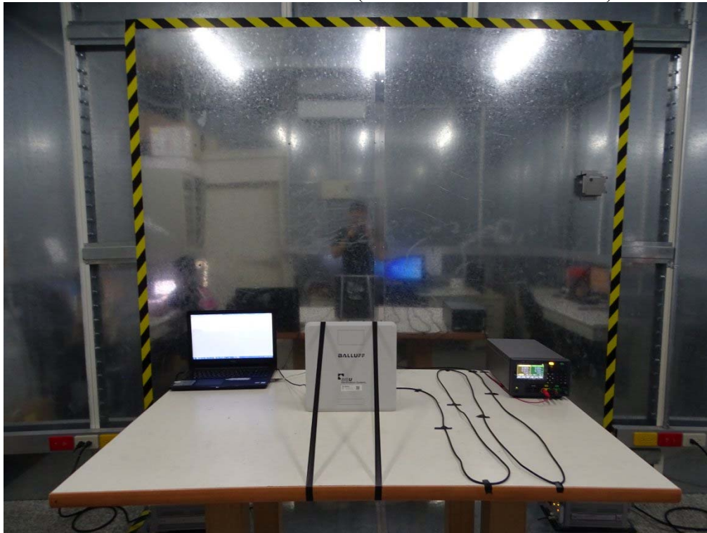
Front View of Conducted Test (BIS U-620-068-111-00-ST29)
