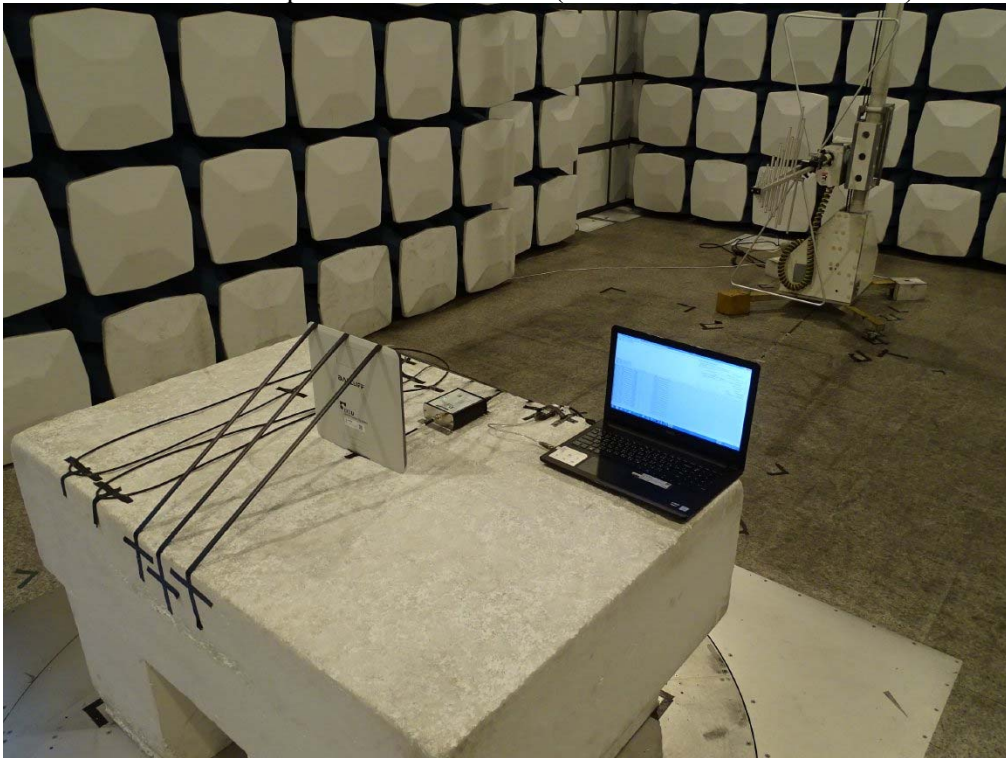
Back View of Spurious Emission Test (BIS U-620-068-111-00-S115)
