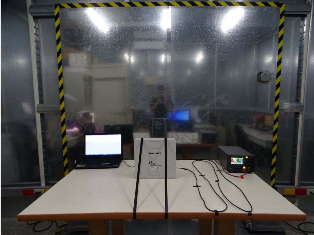
Front View of Conducted Test (BIS U-626-069-111-06-ST31)
