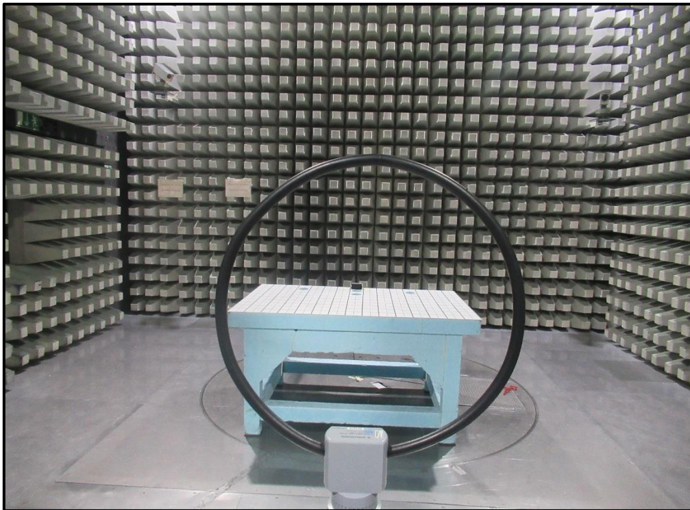
Photo 1 Radiated Test Setup from 9 kHz to 30 MHz – EUT with Ferrite antenna (BIS VM-351-401-S4)
