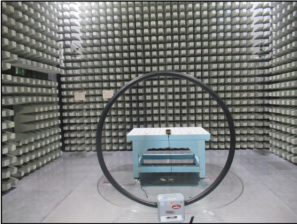
Photo 3 Radiated Test Setup from 9 kHz to 30 MHz – EUT with PCB antenna (BIS VM-341-401-S4)
