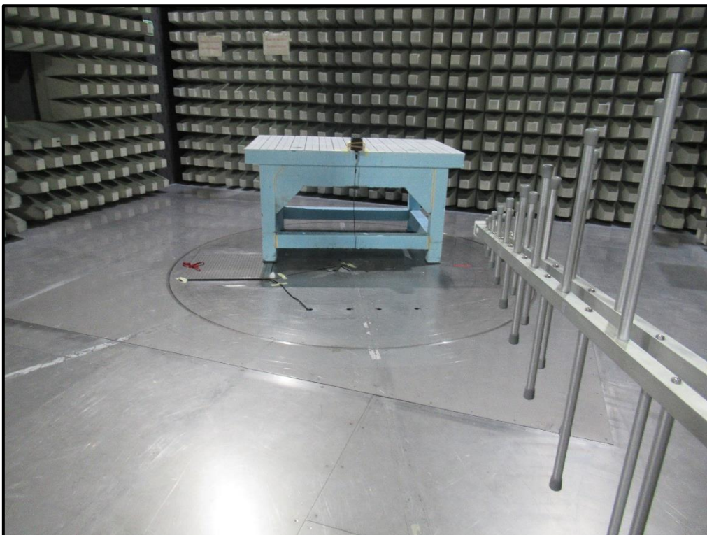
Photo 8 Radiated Test Setup from 30 MHz to 1 GHz – EUT with PCB antenna (BIS VM-341-401-S4)
