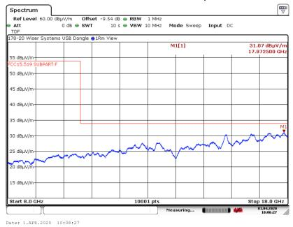
6.5.14. 8 to 18 GHz Vertical at 1 Meter, 6.8 Mbps - 16M
