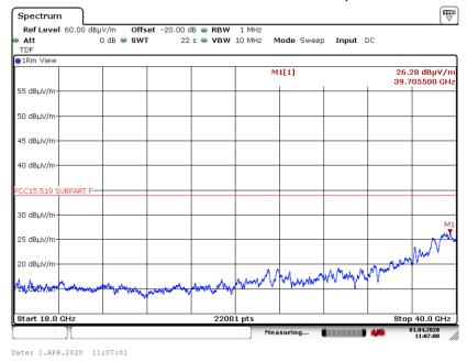
6.5.18. 18 to 40 GHz Vertical at 0.3 Meter, 110 kbps - 16M
