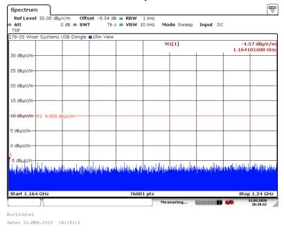
6.6.3.2 Vertical Measurement Polarity 1164 to 1240 MHz
