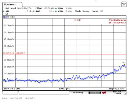
6.5.20. 18 to 40 GHz Vertical at 0.3 Meter, 110 kbps - 64M
