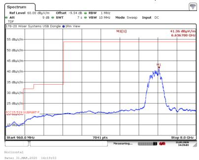
6.5.4. 960 MHz to 8 GHz Vertical at 1 Meter, 110kbps - 64M
