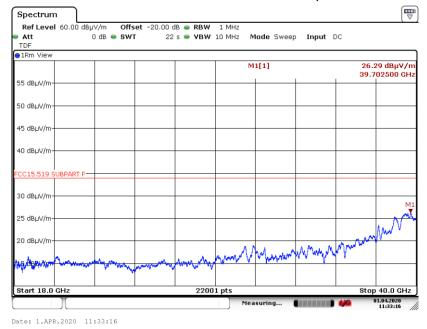
6.5.22. 18 to 40 GHz Vertical at 0.3 Meter, 6.8 Mbps - 16M
