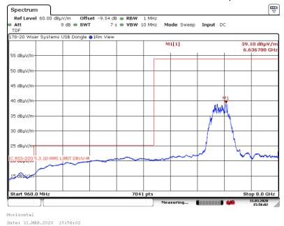
6.5.32. 960 MHz to 8 GHz Vertical at 1 Meter, 6.8 Mbps - 64M
