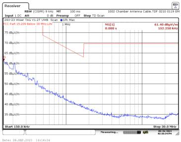
6.4.1.8 Perpendicular Measurement Antenna – 150 kHz to 30 MHz – CH3 Normal
