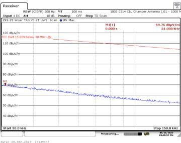
6.4.1.2 Perpendicular Measurement Antenna – 30 to 150 kHz – CH3 Normal
