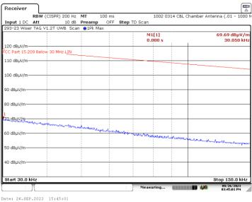
6.4.1.4 Parallel Measurement Antenna – 30 to 150 kHz – CH3 Wide
