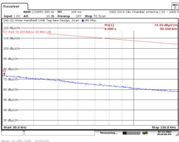
6.4.1.26 Perpendicular Measurement Antenna – 30 to 150 kHz – Z Axis CH5 16M
