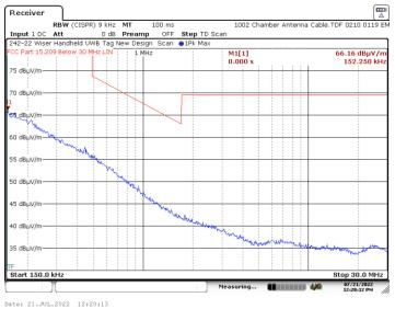
6.4.1.35 Perpendicular Measurement Antenna - 150 kHz to 30 MHz - Z Axis CH2 16M
