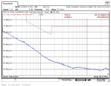
6.4.1.33 Ground Parallel Measurement Antenna - 150 kHz to 30 MHz - Y Axis CH2 16M
