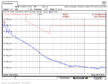
6.4.1.45 Ground Parallel Measurement Antenna - 150 kHz to 30 MHz - Z Axis CH4 16M
