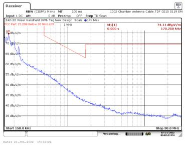
6.4.1.37 Parallel Measurement Antenna - 150 kHz to 30 MHz - X Axis CH4 16M
