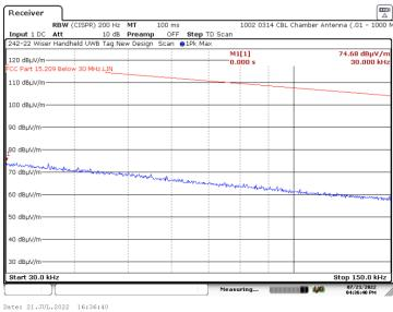
6.4.1.2 Perpendicular Measurement Antenna - 30 to 150 kHz - X Axis CH2 16M
