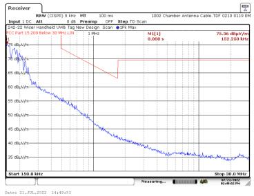
6.4.1.43 Parallel Measurement Antenna - 150 kHz to 30 MHz - Z Axis CH4 16M
