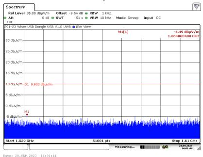
6.6.3.6 Vertical Measurement Polarity 1559 to 1610 MHz, CH3 Normal
