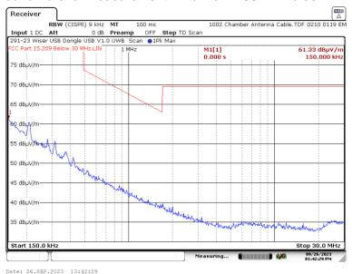
6.4.1.10 Parallel Measurement Antenna – 150 kHz to 30 MHz – CH3 Wide
