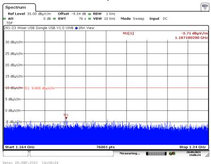
6.6.3.2 Vertical Measurement Polarity 1164 to 1240 MHz, CH3 Normal
