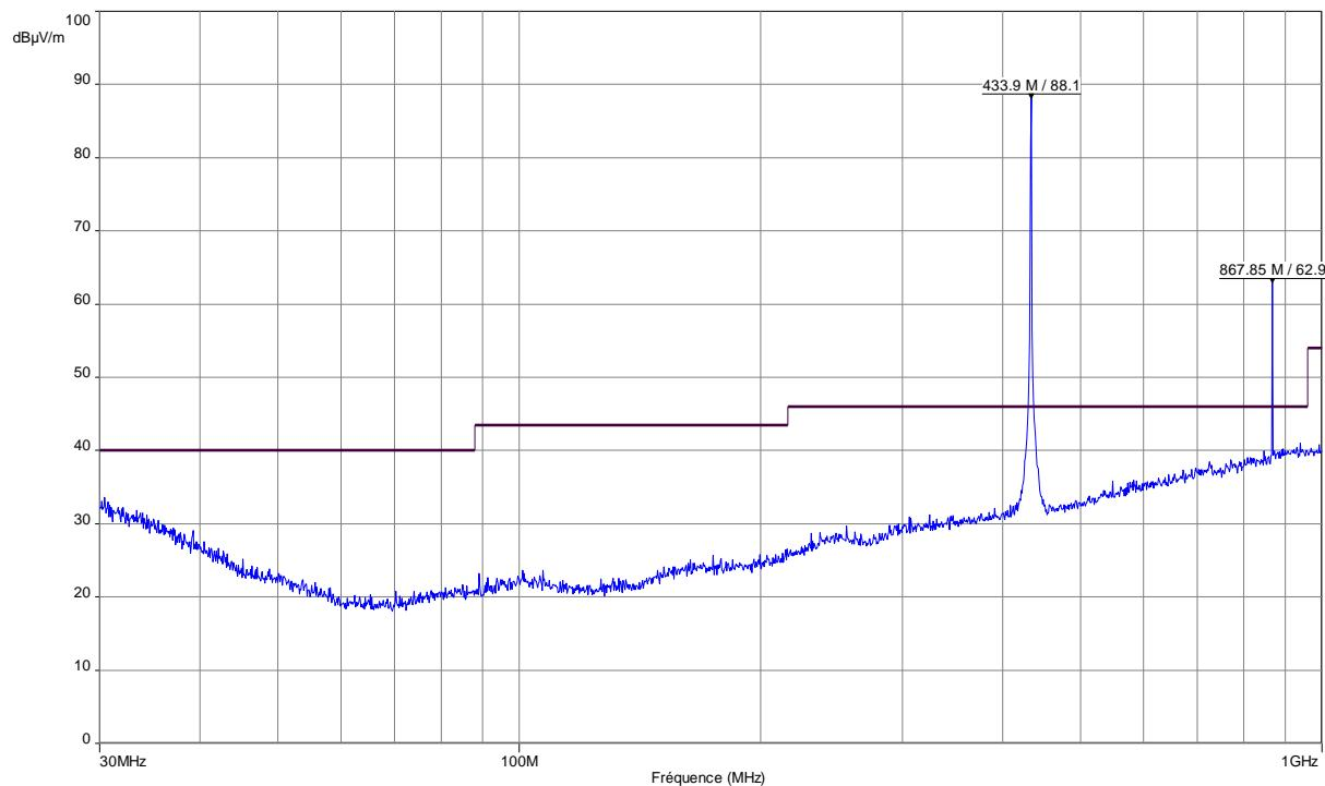
Note: Pre-scan graph only for identification purpose. 433,92MHz frequency observed is the carrier frequency.
