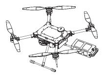
2. Insert one end of the battery into the battery holder, and press the other end upward. When a "click" sound is heard, gently pull the battery outward to confirm if the battery is loose:
