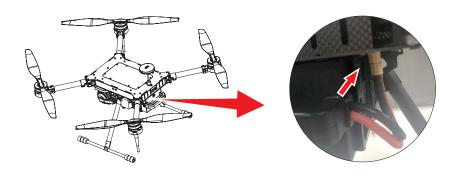
• Note: Make sure the drone power switch is in a off (OFF) state when installing the battery.
