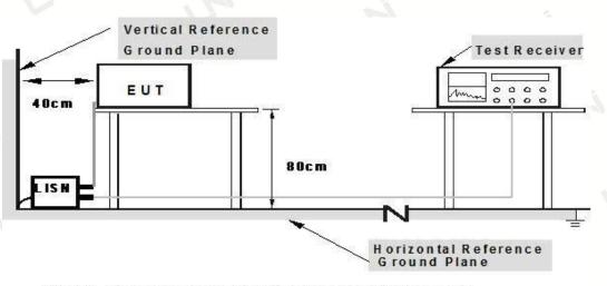
Note: 1.Support units were connected to second LISN. 2.Both of LISNs (AMN) are 80 cm from EUT and at least 80 from other units and other metal planes
