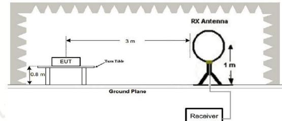
2. Radiated Emission Test-Up Frequency 30MHz~1GHz
