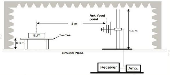
3. Radiated Emission Test-Up Frequency Above 1GHz
