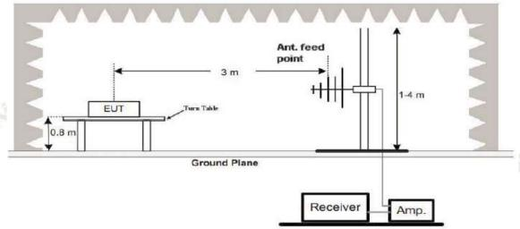
3. Radiated Emission Test-Up Frequency Above 1GHz
