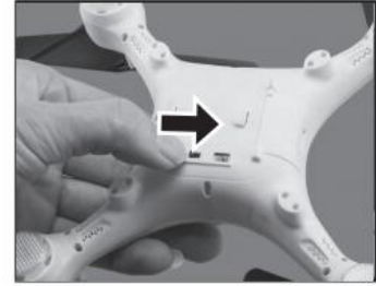
Step 3: Close the battery cover and turn on the quadcopter.
