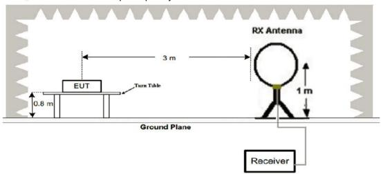
2. Radiated Emission Test-Up Frequency 30MHz~1GHz
