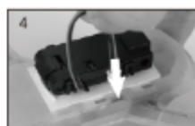
connect connecting line of camera with power supply socket of fuselage's camera.
