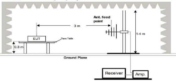
3. Radiated Emission Test-Up Frequency Above 1GHz
