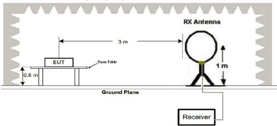
2. Radiated Emission Test-Up Frequency 30MHz~1GHz
