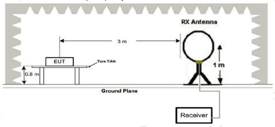
2. Radiated Emission Test-Up Frequency 30MHz~1GHz
