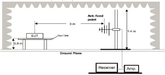
3. Radiated Emission Test-Up Frequency Above 1GHz
