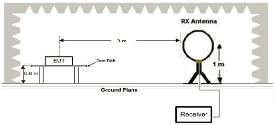
2. Radiated Emission Test-Up Frequency 30MHz~1GHz
