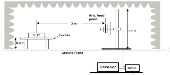
3. Radiated Emission Test-Up Frequency Above 1GHz
