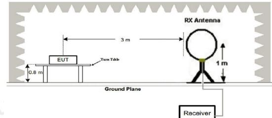
2. Radiated Emission Test-Up Frequency 30MHz~1GHz
