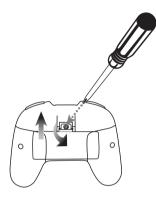
Use screwdriver (not included) and remove battery cover.
