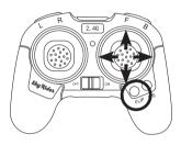
Press the **Flip button,** then move the **Right Control Stick** in any direction.
