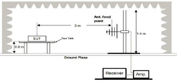
3. Radiated Emission Test-Up Frequency Above 1GHz
