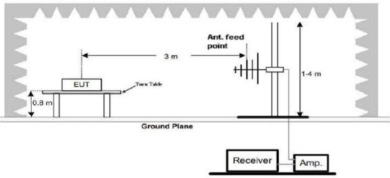
3. Radiated Emission Test-Up Frequency Above 1GHz
