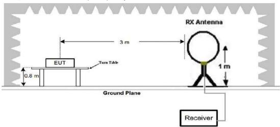
2. Radiated Emission Test-Up Frequency 30MHz~1GHz
