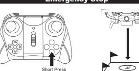
Note: The emergency stop function can be only used in case of emergency during the flight to avoid any of damage or injury. For any reason, if you need to stop the drone, press the "Emergency Stop" button or pull the left joystick down to the lowest, the drone will stop the propellers from spinning. Be sure the ground is clear of any objects as this will command the rotor to shut down and crash land.
