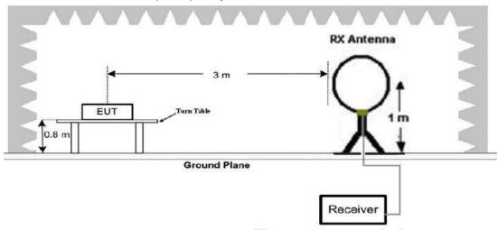
2. Radiated Emission Test-Up Frequency 30MHz~1GHz
