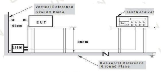
Note: 1. Support units were connected to second LISM. 2.Both of LISMs (AMM) are 80 cm from EUT and at least 80 from other units and other metal planes
