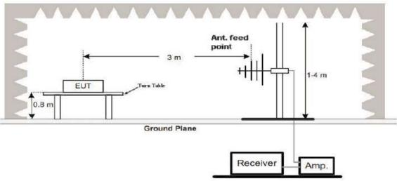
3. Radiated Emission Test-Up Frequency Above 1GHz
