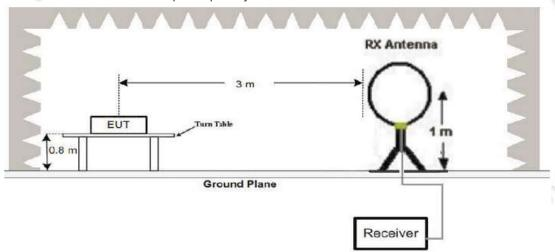
2. Radiated Emission Test-Up Frequency 30MHz~1GHz
