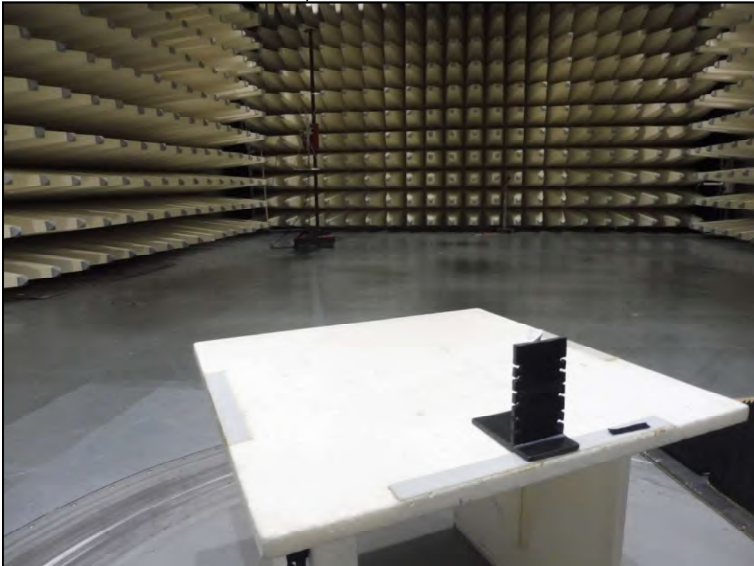
Photo 2: setup of radiated emission > 1 GHz
