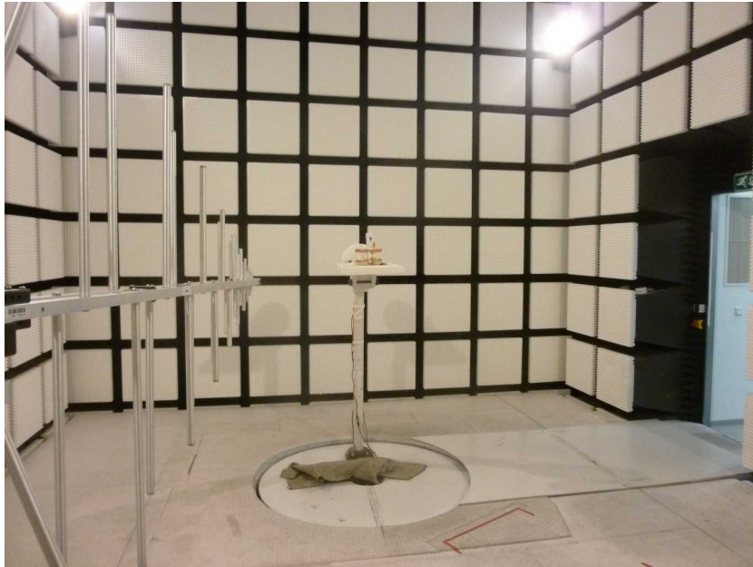
Photo 7: EUT at the anechoic chamber
