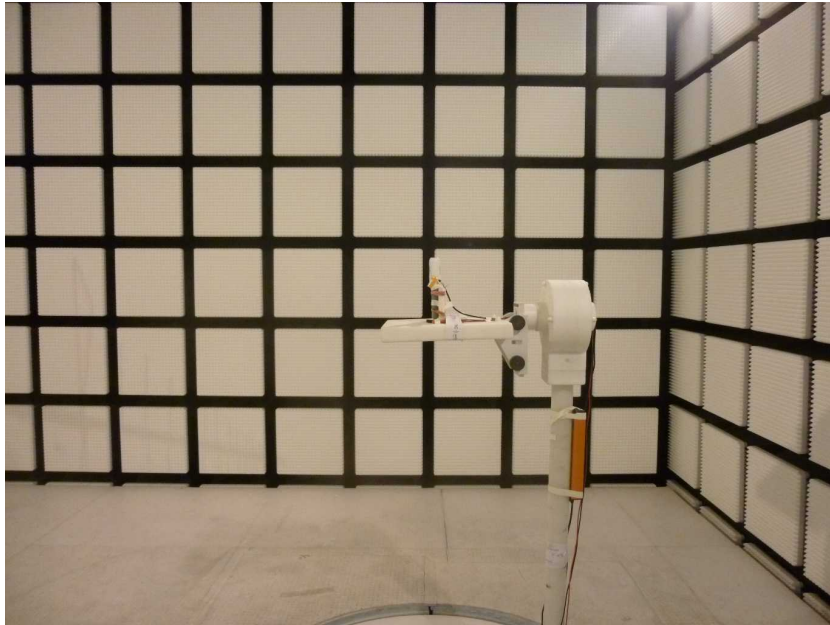
Photo 5: EUT at the anechoic chamber
