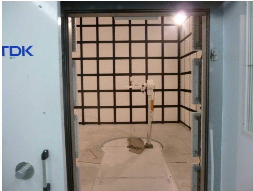
Photo 1: EUT at the anechoic chamber
