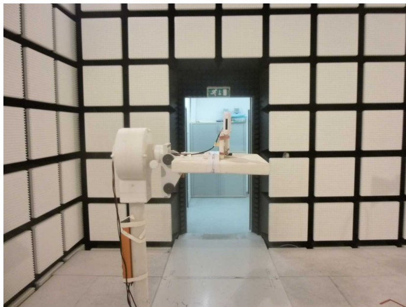
Photo 2: EUT at the anechoic chamber
