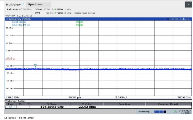
Low Channel, 160 MHz Bandwidth, Vertical
