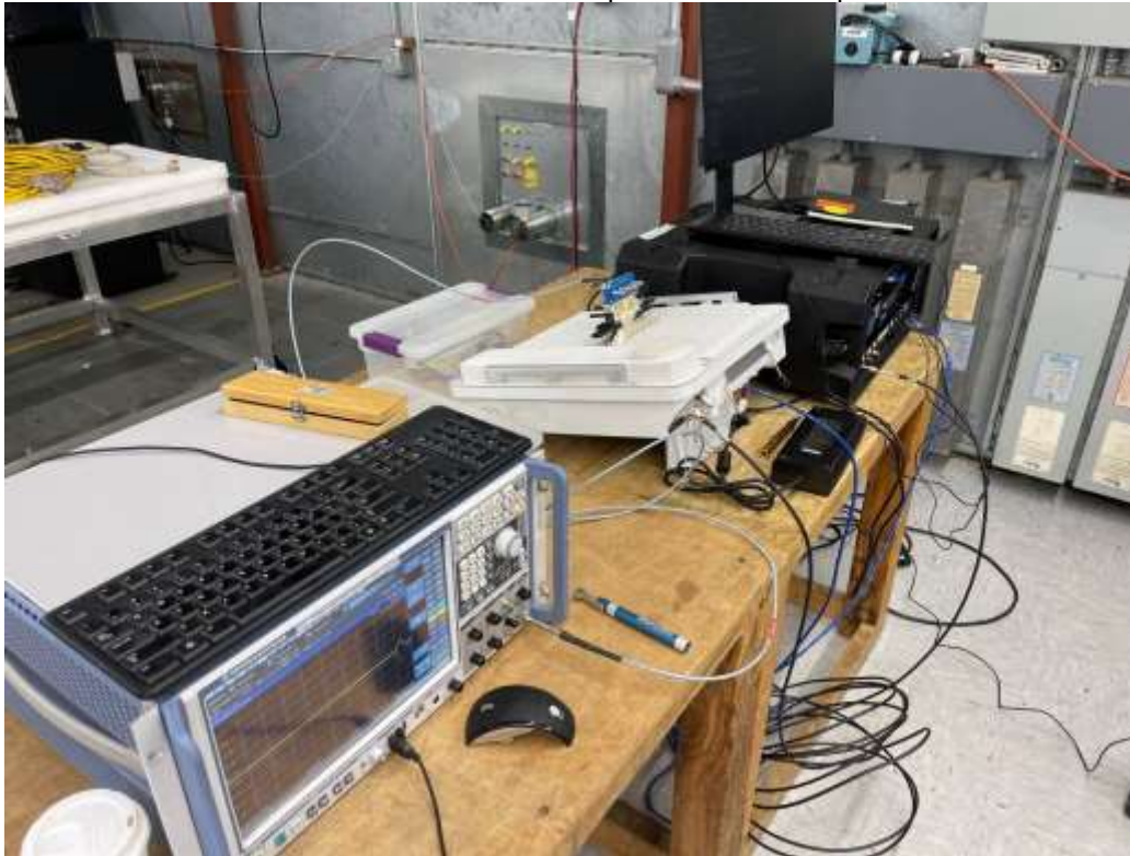
Conducted Power and Spurious Test Setup
