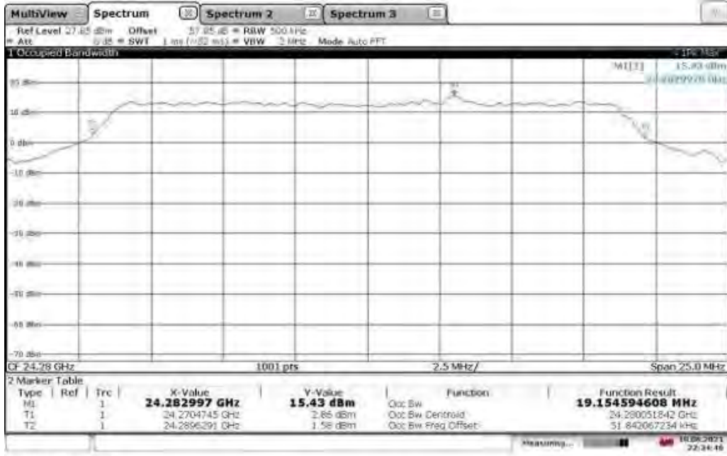
Occupied Bandwidth (Vertical Polarity) – S01411_24.28GHz_BW20M_MCS8_Path 3
