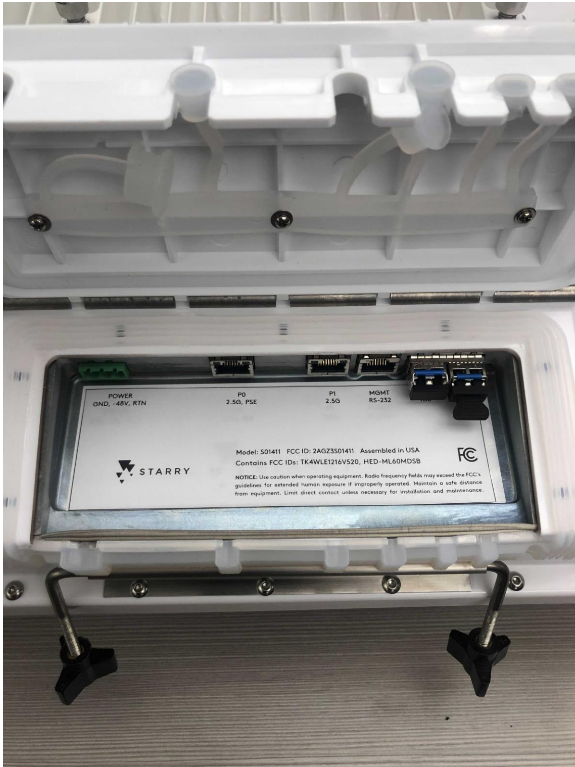
Figure 5. TITAN 24 RF, Connector Panel Interface
