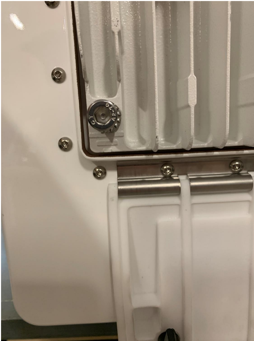
Figure 3. Grounding, External, Rear Assy View
